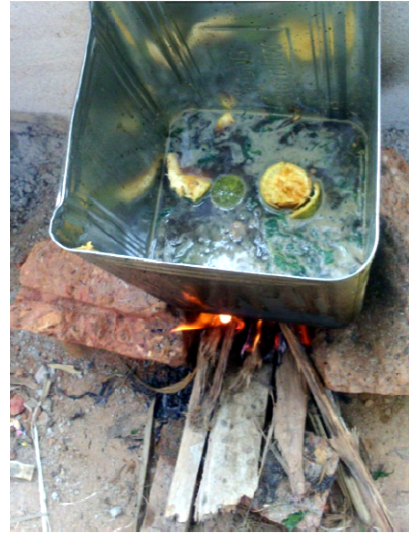
Figure 9: Boiling of the traditional binder to add in Surkhi Mortar
